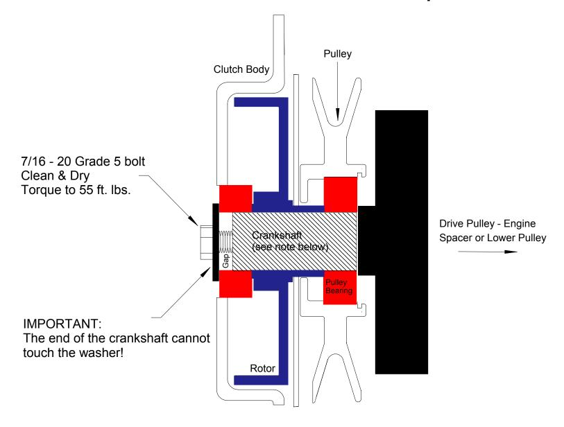
Note: Crankshaft MUST have contact with both bearings.
