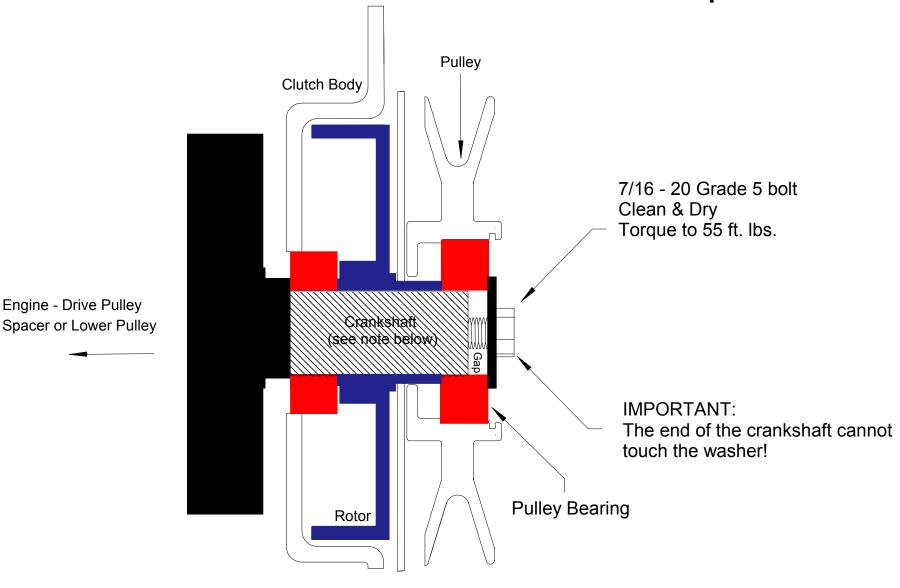
Note: Crankshaft MUST have contact with both bearings. If the crankshaft is too short and does not enter into the second bearing the clutch will fail.
